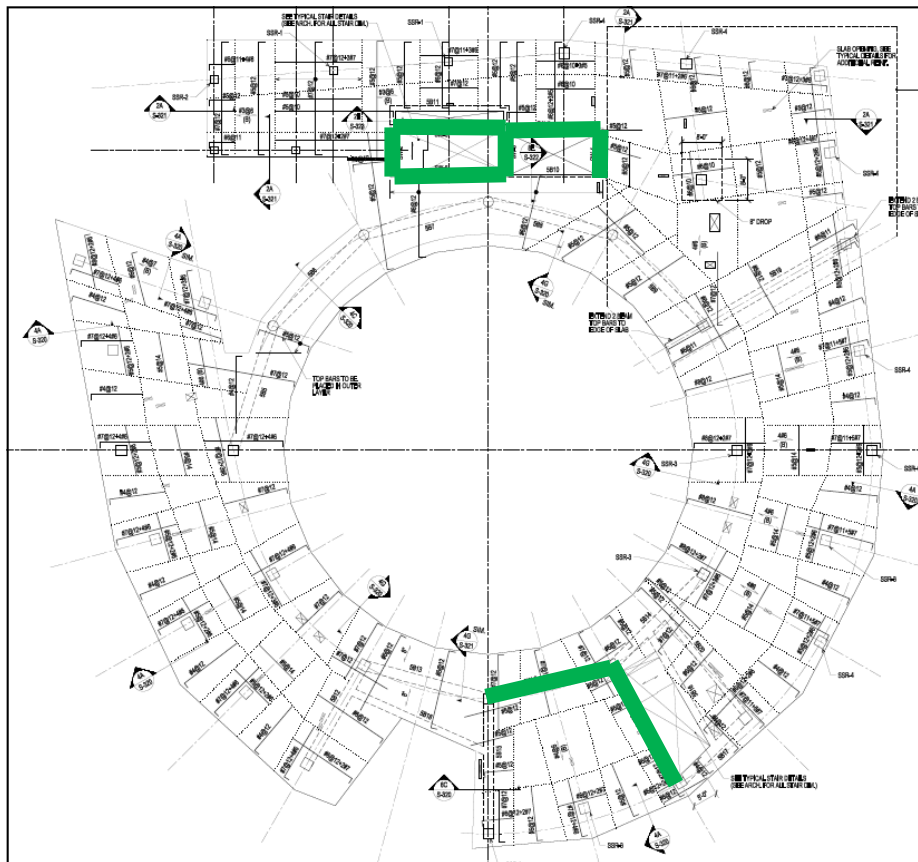
Figure 3: Shear wall locations. Courtesy of RTKL.
